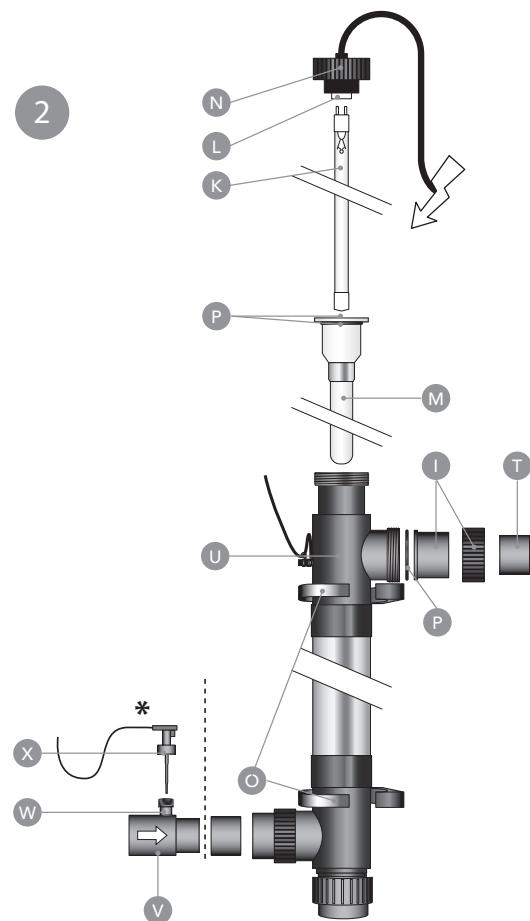
\* Flow switch. Only for TECH UV-C 130W.
